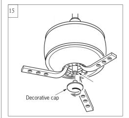
Install a decorative cap onto motor shaft by turning clockwise until tight.
