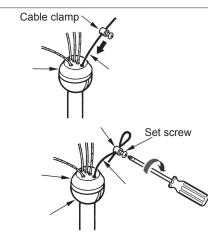
Install cable clamp. Cable clamp provided.
