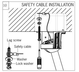
For Canadian installation and for USA fan and light kit combinations over 35 lbs, in both flush and downrod modes the safety cable must be installed into the house structure beams using 1.5" lag screws, washers and lock washers provided. Make sure that when the safety cable is fully extended the lead wires are longer than the cable and no stress is placed on the lead wires.
