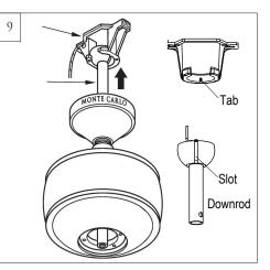
Install ball end of downrod into mounting bracket opening. Align (engage) slot on ball with tab on mounting bracket. **Warning:** Failure to align slot on ball with tab may result in serious injury.
