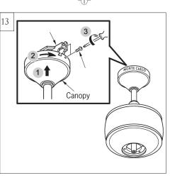
Raise canopy to mounting bracket, aligning loosened screws in mounting bracket with slotted holes in canopy. Twist canopy to lock. Reinstall the screws removed in step 12 and tighten all screws securely.
