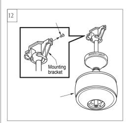
Partially loosen 2 of the set screws on mounting bracket corresponding to the slotted holes on the canopy upper ring. Remove the other 2 set screws. Save screws.
