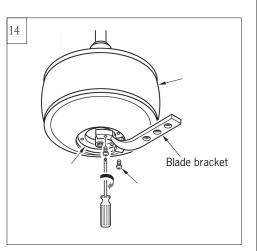
Install blade bracket onto motor with set screws provided.
