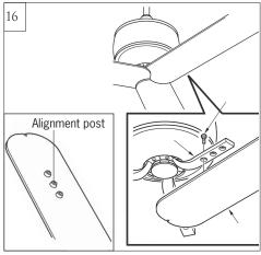
Install blade, aligning 3 alignment posts on blade with the holes in blade bracket, then install it with set screws provided. Repeat this process for remaining blades. Tighten all screws securely.
