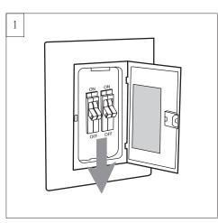
Before you begin installing the fan, Switch power off at Service panel and lock service disconnecting means to prevent power from being switched on accidentally. When the service disconnecting means cannot be locked, securely fasten a warning device, such as a tag, to the service panel.
