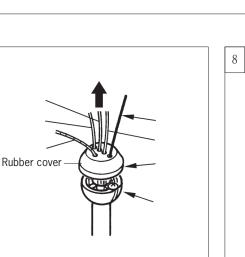
Thread lead wires, grounding wire and safety cable through watertight rubber cover, then place the rubber cover onto hanger ball on downrod. Rubber cover provided.
