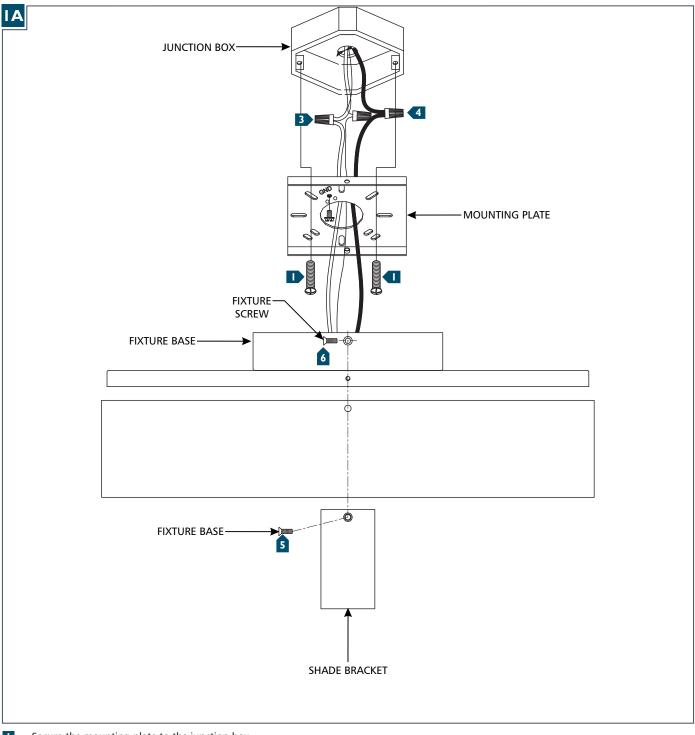
Secure the mounting plate to the junction box.
