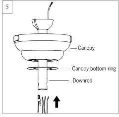
Place downrod over canopy and canopy bottom ring. Thread lead wires and safety cable from motor assembly through downrod.
