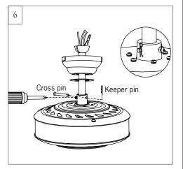
Slip downrod into motor housing yoke, aligning holes and install cross pin and keeper pin.
