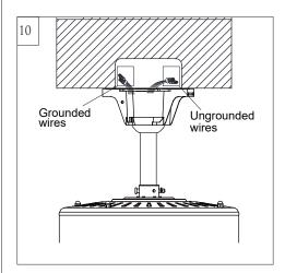
After making the wire connections, the wires should be spread apart with the grounded conductor and the equipment-grounding conductor on one side of the outlet box and ungrounded conductor on the other side of the outlet box. The splices after being made should be turned upward and pushed carefully up into the outlet box.
