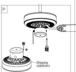
Remove shipping stabilizers from motor assembly.
