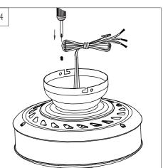
Reinstall the 3 set screws remove in step 12. Tighten screws securely.
