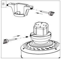
Install 2 of the screws to the side panel of mounting bracket corresponding to the open slotted holes on the canopy upper rim, screws provided. Remove the thread studs from the lower part of the mounting bracket.
