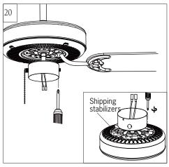
Remove shipping stabilizers from motor assembly.
