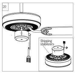
Remove shipping stabilizers from motor assembly.
