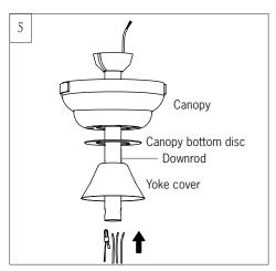
Place downrod over canopy, canopy bottom disc and yoke cover. Thread lead wires and safety cable from motor assembly through downrod.
