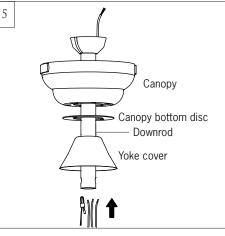
Place downrod over canopy, canopy bottom disc and yoke cover. Thread lead wires and safety cable from motor assembly through downrod.
