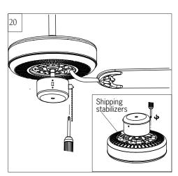
Remove shipping stabilizers from motor assembly.
