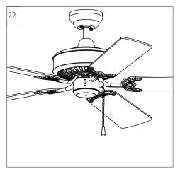
Install fan pull chain to preassembled pull chain on fan. Pull chain provided.
