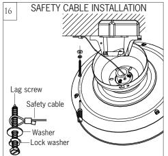
For Canadian installation and for USA fan and light kit combinations over 35 lbs, in both flush and downrod modes the safety cable must be installed into the house structure beams using 3" lag screws, washers and lock washers provided. Make sure that when the safety cable is fully extended the lead wires are longer than the cable and no stress is placed on the lead wires.
