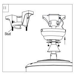
Lift Canopy allowing the 2 studs to protrude through the canopy. Next lift the cover ring and install knurled nuts as shown. Tighten the knurled nuts securely. The canopy should adjust for any irregularity in the ceiling or Outlet box.
