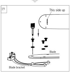
Install blade bracket with blade by 3 blade screws and washers provided. Tighten screws securely. Repeat this process for remaining blades. **Note**: Make sure the side with a label "This side up" is installed upward.
