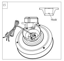
To prepare the fan for wiring, hang fan onto mounting bracket by sliding the canopy over the mounting bracket hook (**Use one of non-slotted holes on the rim of the canopy**).
