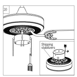
Remove shipping stabilizers from motor assembly.
