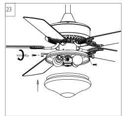
Partially loosen 3 set screws from light fixture.
