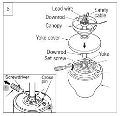
Partially loosen downrod set screws from yoke at top of motor assembly. Thread lead wires and safety cable from motor assembly through downrod. **Helpful hint:** For easy assembling of the cross pin on the next installation step. After slip downrod into the motor yoke, carefully insert a Phillips screwdriver through the yoke and downrod (**don't damage the lead wires**) as a guide and then push the cross pin and pull the screwdriver in the meantime as shown in the inset.
