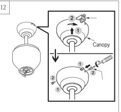
Raise canopy to mounting bracket, aligning loosened screws in mounting bracket with slotted holes in canopy. Twist canopy to lock. Reinstall the screws removed in step 11 and tighten all screws securely.
