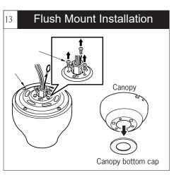
Remove every other screws (the screws located at round holes) from yoke located on top of fan assembly. Keep screws. Remove canopy bottom cap from canopy.
