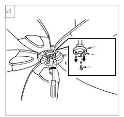
Loosen 2 and remove 1 preassembled set screws from the plate on motor. Save screw for later use.
