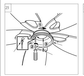
Attach light fixture onto the light plate, aligning keyhole slots on the light fixture with the preassembled set screws on light plate and twist clockwise until lock. Reinstall the screw removed in step 23. Tighten all screws securely.
