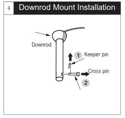
Remove preassembled keeper pin and cross pin from downrod.
