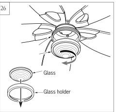
Place glass over glass fixed ring, aligning the thread on light fixture and attach it onto light fixture by turning clockwise till tight.
