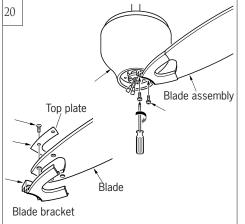
Align the holes of blade bracket, blade and the top plate of blade bracket. Install blade bracket with blade by 4 blade screws provided. Tighten screws securely. Repeat this process for remaining blades. Install the blade assembly to motor using the set screws provided. Tighten screws securely
