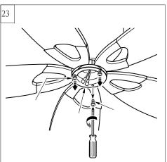
Loosen 2 and remove 1 preassembled set screws from the light plate. Save screw for later use.
