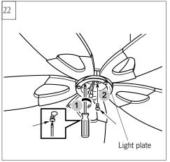
Attach light plate onto the plate on motor, aligning its keyhole slots with the preassembled set screws on the plate and twist clockwise till lock. Reinstall the screw removed in step 21. Tighten all screws securely.
