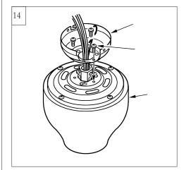
Place canopy over lead wire and safety cable and align the larger holes in canopy with the set screws on yoke. Reinstall the 3 set screws remove in step 13. Tighten screws securely.
