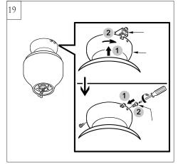
Raise canopy to mounting bracket, aligning loosened screws in mounting bracket with slotted holes in canopy. Twist canopy to lock. Reinstall the screws removed in step 18 and tighten all screws securely.
