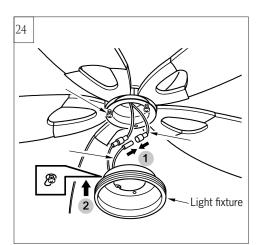
Connect white wire from fan to white wire from light fixture, and then connect blue (or black) wire from fan to blue (or black) wire from light fixture.
