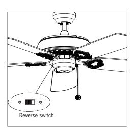
Setting the reverse switch in the left hand side will result in downward airflow and setting the switch in the right hand side will result in upward airflow.
