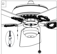
Connect the quick connectors from fan and switch housing. Make sure quick connectors are clasped firmly. Install the switch housing onto the top plate, aligning the keyhole slots on the switch housing with the preassembled screws on top plate and twist it clockwise till lock. Reinstall the set screw removed in step 21 and tighten all screws securely.
