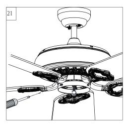
Loosen 2 and remove 1 preassembled screw from top plate of switch housing.
