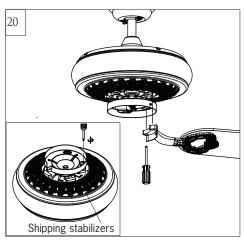
Remove shipping stabilizers from motor assembly.
