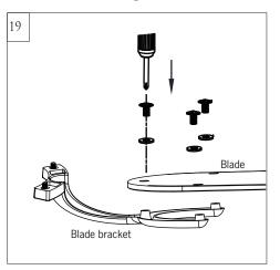
Install blade bracket with blade by 3 blade screws and washers provided. Tighten screws securely. Repeat this process for remaining blades.
