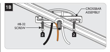
**Note:** If necessary, loosen the nut on the crossbar to adjust it to the desired position.
