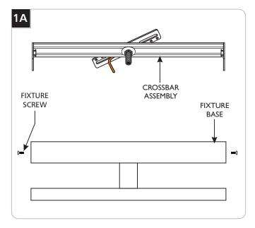
1 Separate the crossbar assembly from the fixture base by unscrewing and removing the two fixture screws.
