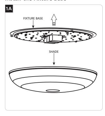
1 Separate the shade from the fixture base by rotating the shade out of the fixture base.
