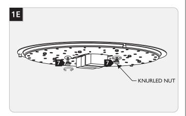
Properly place all wires and wire nut connections into the junction box, mount the fixture base to the ceiling by reinstalling it onto the mounting plate, and secure it tightly with the knurled nuts.
