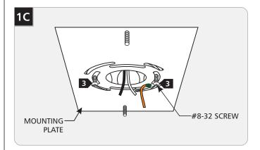
3 Secure the mounting plate to the junction box with 2 #8-32 screws.
