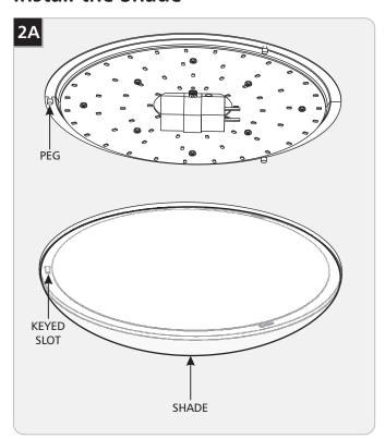
Align the pegs on the mounting plate with the keyed slots on the shade, push the shade onto the pegs, and rotate it to secure in place.
