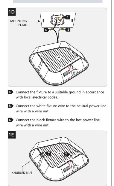
Mount the fixture base to the ceiling by reinstalling it onto the mounting plate and secure it tightly with the knurled nuts.
