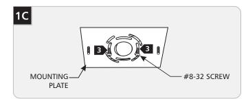
Secure the mounting plate to the electrical box with 2 #8-32 screws.
