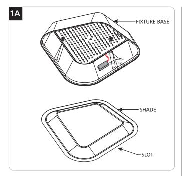
Insert a flat head screw driver into the slot on the shade and separate the shade from the fixture base.
