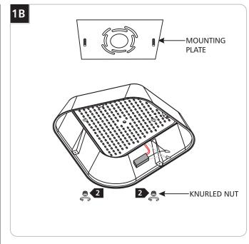
Remove the mounting plate from the fixture base by unscrewing the two knurled nuts.
