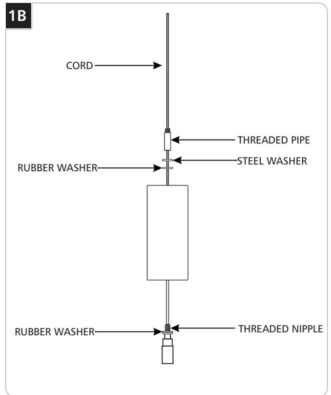
**2** Feed the cord through the inner shade and ensure that the rubber washer is seated properly on the threaded nipple.
