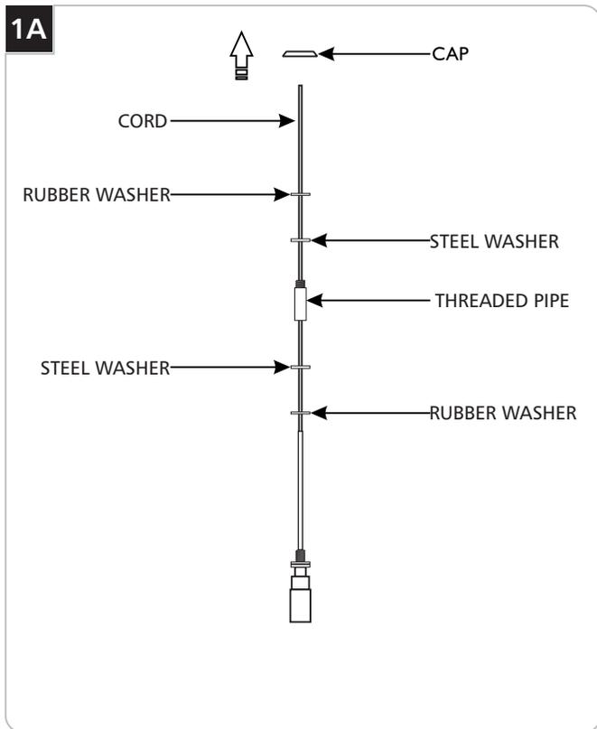
**1** Remove the cap, rubber washer, steel washer, threaded pipe, steel washer, and rubber washer from the cord.
