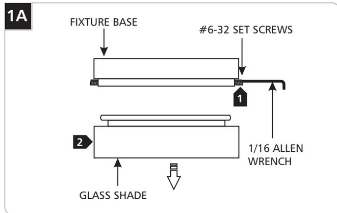
**1** While supporting the glass shade, loosen (**Do Not Remove**) the four #6-32 set screws on fixture base with the 1/16 Allen wrench.
