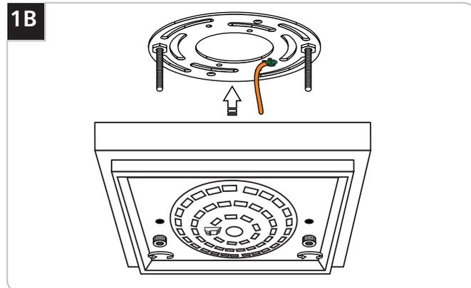
**3** Remove the mounting plate from the fixture base by unscrewing the two knurled nuts.
