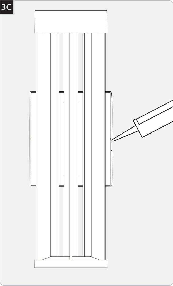
8 For wet locations, caulk around the base with waterproof construction sealant.
