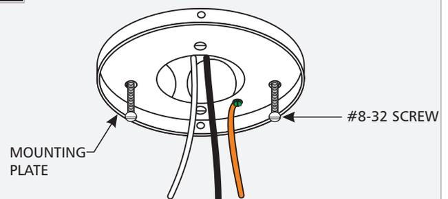
**2** Secure the mounting plate to the electrical box with the two #8-32 screws provided.
