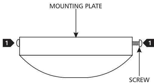
**1** Separate the mounting plate from the canopy by removing the two screws.
