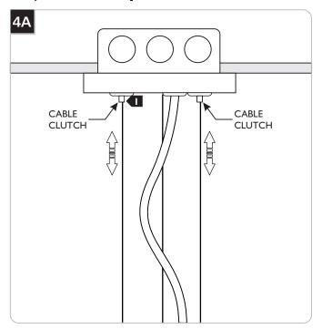
1 If necessary, adjust the aircraft cables until the fixture is level; feed the cable into the cable clutch to raise the fixture and push in on the cable clutch nipple to release the cable and lower the fixture.
