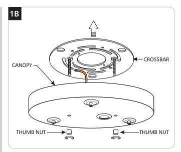
4 Remove the crossbar from the assembly by unscrewing the two thumb nuts.
