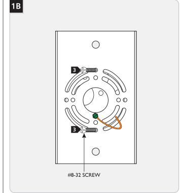
Attach the mounting plate to the electrical box using the two provided #8-32 screws.
