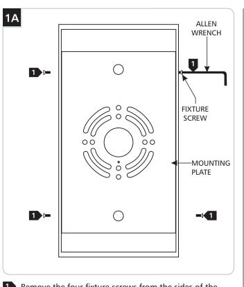
Remove the four fixture screws from the sides of the fixture using the provided Allen wrench.
