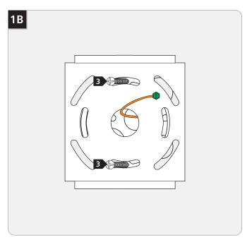
Attach the mounting plate to the electrical box using the two provided #8-32 screws.
