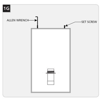
14 With the allen wrench, tighten the set screws to secure the fixture to the mounting plate.
