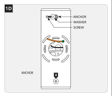
Slide a #8 screw through a washer, and screw it into an anchor to secure the fixture base to the wall. Repeat for the other anchor.
