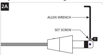
1 Back out (do not remove) the set screw on tip of the connector with the provided Allen wrench.
