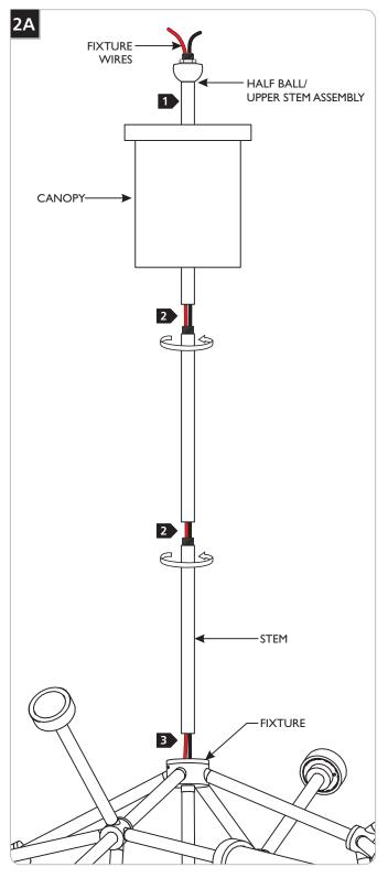
Feed the half ball/upper stem assembly through the top of the canopy.
