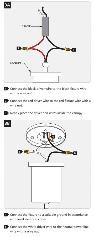
6 Connect the black driver wire to the hot power line wire with a wire nut.
