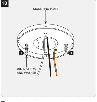
Secure the mounting plate to the electrical box with the two washers and #8-32 screws provided.
