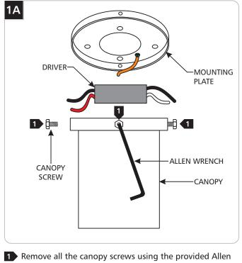
Remove all the canopy screws using the provided Allen Wrench.
