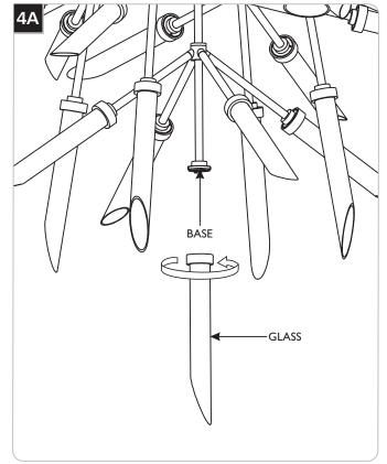
Install the glass by screwing it into the base. Do not over-tighten.
