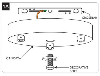
Remove the crossbar from the canopy by completely unscrewing the decorative bolt.
