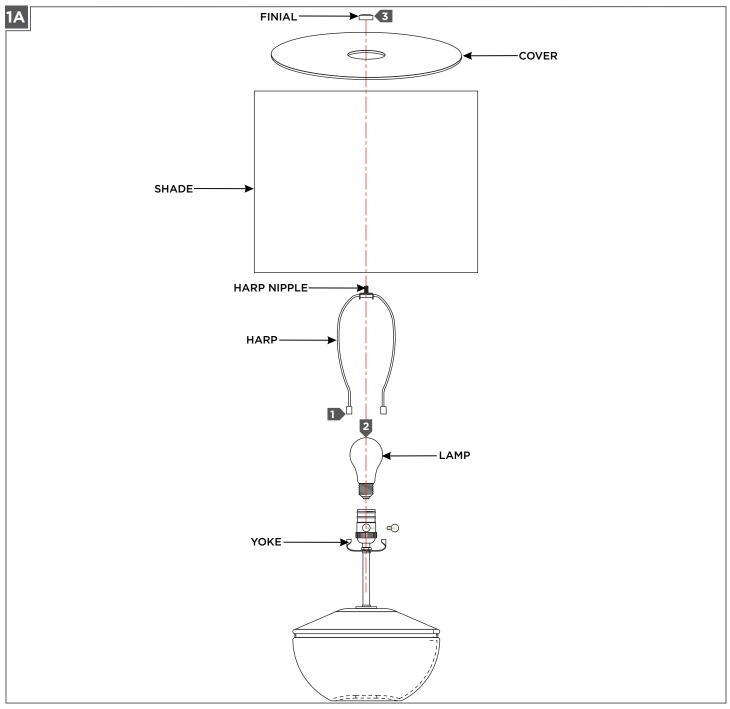
**1** Install the harp by inserting into the yoke.
