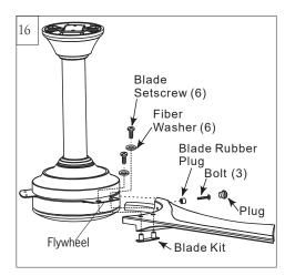
Engage the blade with flywheel, aligning the holes and then partially install 2 blade set screws and washers from top and one bolt from side of blade as shown. Repeat this process for remaining blades. Tighten all set screws and bolts securely after all the blade assemblies are installed to flywheel.
