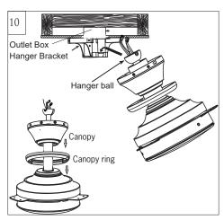
Place canopy ring and canopy over downrod with column. Handle it carefully to avoid damage from scratch. Install ball end of downrod into mounting bracket opening. To slip hanger ball into mounting bracket by slanting fan assembly for about 35 degree as shown in above illustration.
