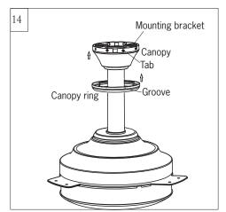
Raise canopy to mounting bracket, aligning loosened screws in mounting bracket with slotted holes in canopy. Twist canopy clockwise to lock. Reinstall screws (with washers) that were previously removed in step 3 and then tighten all screw securely Install canopy ring onto canopy by aligning the grooves in canopy ring with the tabs on canopy and pop it onto canopy.
