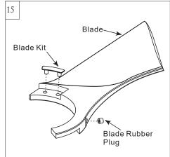
Insert the blade kit and blade rubber plug in position as shown.
