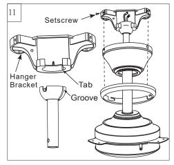
Align (engage) slot on ball with tab on mounting bracket.
