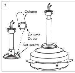
Place column over downrod and put it in position by aligning the recessions with the set screws on top side of housing.
