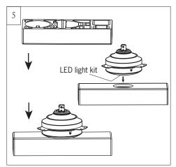
Place fan assembly on styrofoam to keep the LED light kit away from damage and make fan installation easier.
