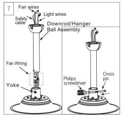
Connect the lead wires and thread safety cable from motor assembly through downrod. **Make sure the plugs are connected securely.**
