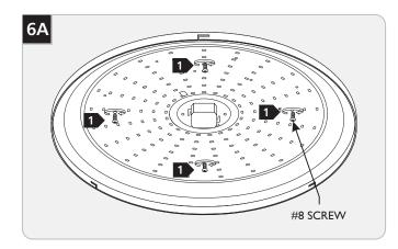
Place the four provided #8 screws in the holes and carefully tighten them to be sure to not damage the LED board.
