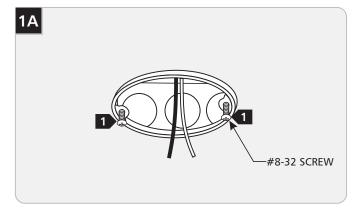
1 Partially screw 2 #8-32 screws. Into the Junction box.
