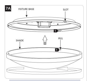
CAUTION: Improperly aligning the pegs before rotating the shade into place may cause damage to slots. Make sure the shade sits flush before rotating.
