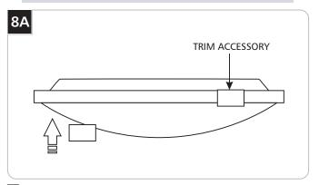
1 Attach the trim accessories to the rim of the shade. Imbedded magnets will allow the accessories to snap into place.
